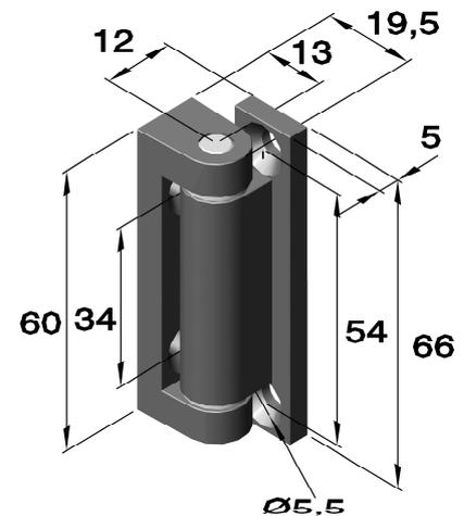
**Art.no.: HS40** (drilled and countersunk)
