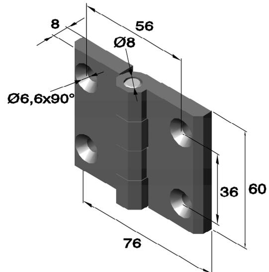
**Art.no.: HF50** (drilled and countersunk)
